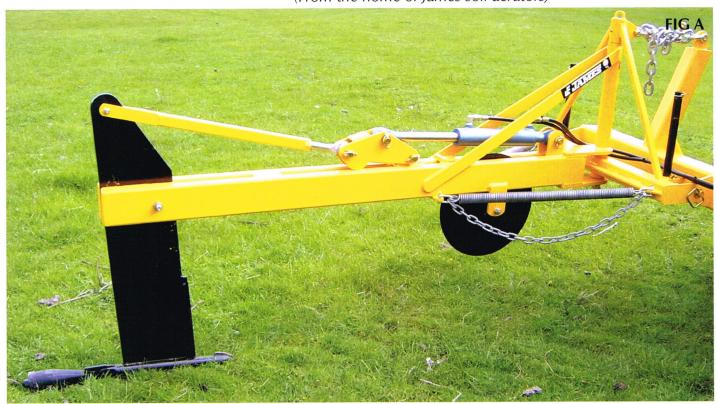
The James Heavy Duty Moleplough is designed to transfer ground water to field tiles or open drains in soils where there is good clay subsoil. The mole plough forms a 60mm channel in the clay at a depth of approximately 46cm providing drainage.
